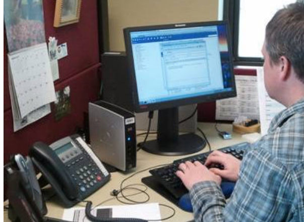
In the new environment, users can log in and access their running applications from any thin client device on the network.
